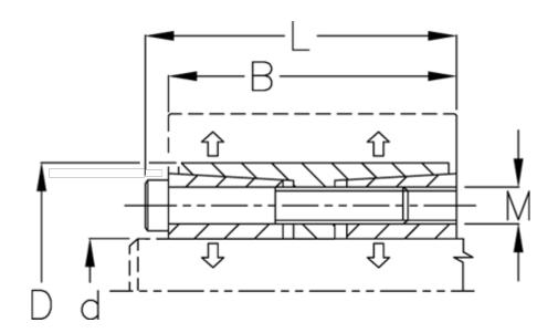
B mm = 54d H8 mm = 45D mm = 75Fit tolerance = Aksel h8, Nav H8
